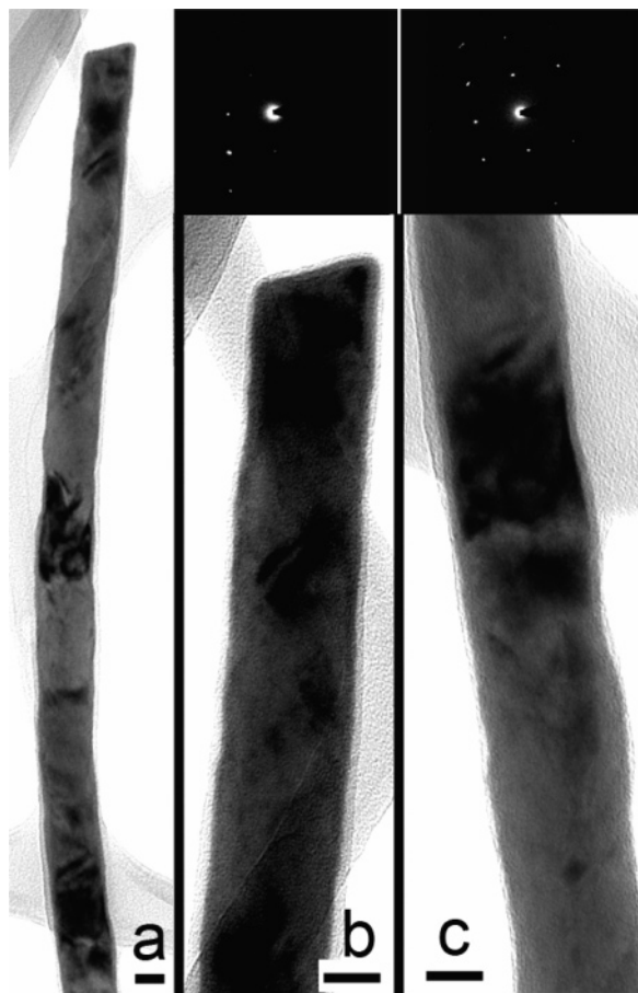
Figure 4. Bright field TEM micrographs of a released nanowire, with corresponding diffraction patterns at two locations along the wire length. Images b and c are from the upper and lower edges of a, respectively. The mottled contrast in the dark areas along the wire length is due to bend contours interacting with localized strained fields. The slight curvature of the nanowire results in a 10^\circ rotation in the diffraction patterns. Scale bars represent 20 nm.
